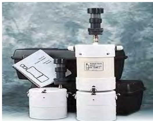
Figure 3: Air Metrics MiniVol sampler
