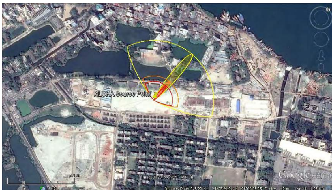
Figure 9-1: Fuel not burning whilst the gas is being dispersed through the pipeline - Flammable area vapor cloud
